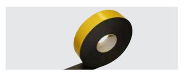
Highly flexible closed cell elastomeric foam (FEF) suitable for hot and cold thermal insulation, featuring a combination of low thermal conductivity, high water vapour diffusion resistance and low flame spread.
